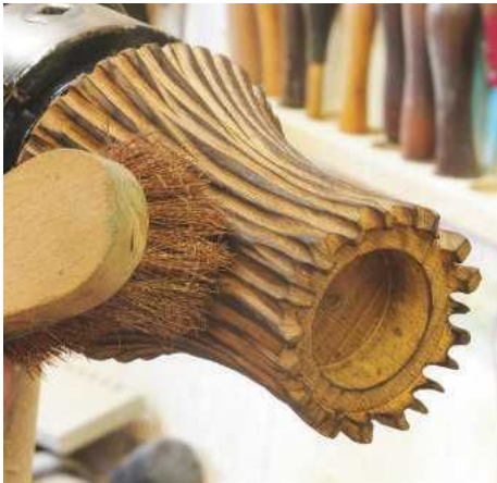
▲ Pic.13 He has given the work a light burn and is now brushing off the carbon with a liming brush. The piece should be very tactile now, looking rough but feeling smooth
